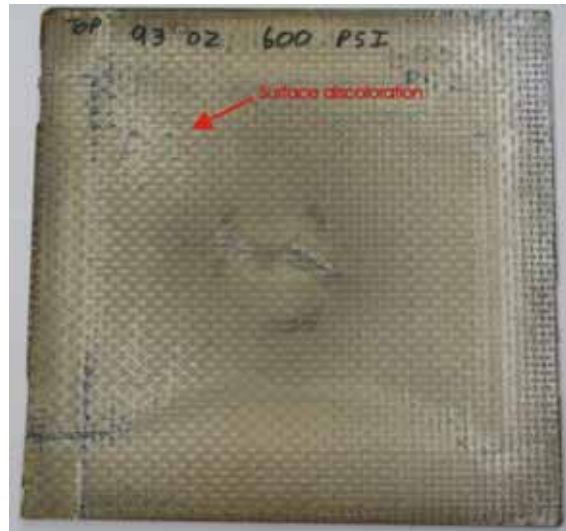
Figure 24. Surface damage to plate subjected to 600 psi input pressure.
