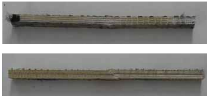
Figure 27. Two forms of failures obtained during compression testing: a) fiber crushing (190 oz) and b) fiber kinking (93 oz).
