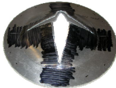
Figure 10. Burst aluminum diaphragm.
