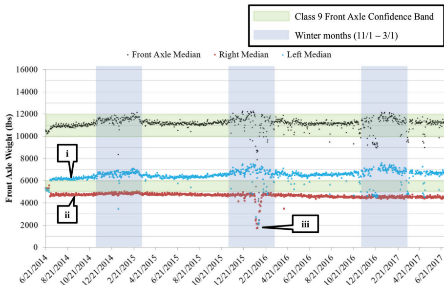
(b) WIM station #953160 lane 1 daily class 9 median front axle data over three years
