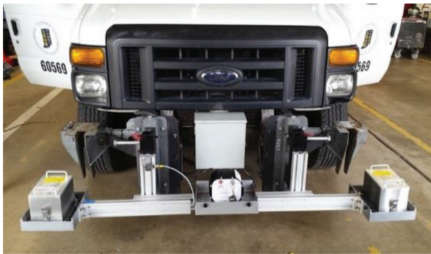
Figure 3.3 Photo of laser setup for acquiring texture data.
