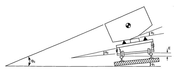
Model for Analyzing Rail Vehicle Response to Track Twist
