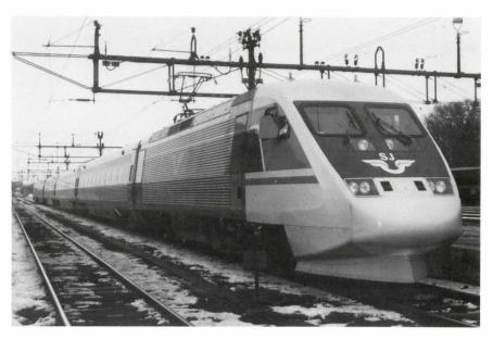
The X2000 Tilting Train: Cab-Car End Forward at a Stop in Sweden Where It Operates over Existing Mixed Traffic Lines at 200 km/h (125 mph)
