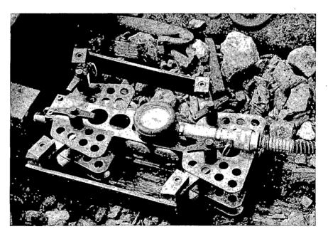
Single Tie Push Test Device for Lateral Resistance Measurement
