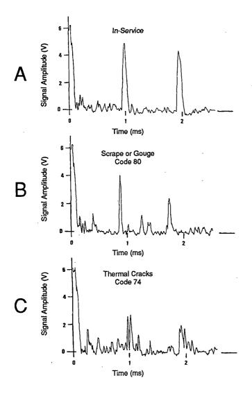
Typical Analog Signals Resulting from Initial Field Evaluations on the Prototype Wheel Crack Detection Unit, Train Speed: 8 km/h (5 mph)
