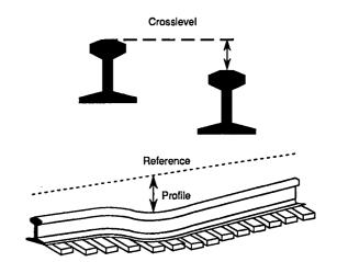
Gauge Geometry and Profile Geometry
