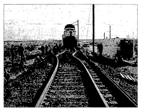
Dynamic Buckling Tests for Buckling Safety Evaluations
