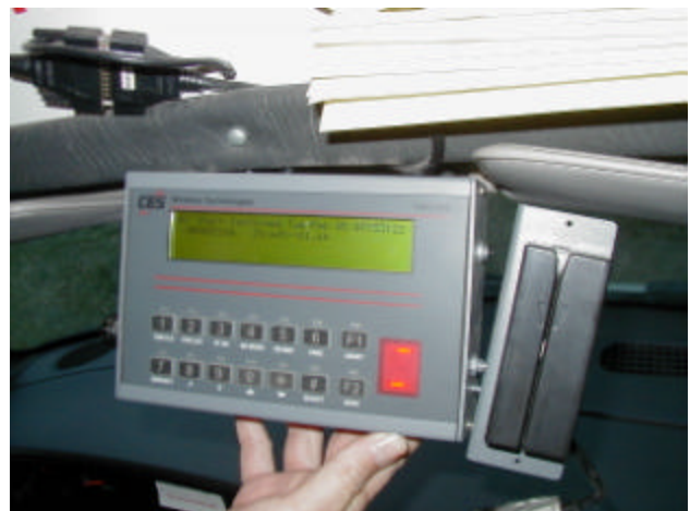
Putnam County’s ITS Deployment included the purchase of 35 new AVL/MDT units with card readers.
