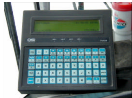
Ottumwa's rural ITS deployment includes MDTs, which are used for communication between drivers and dispatchers and for pre-trip inspections.
