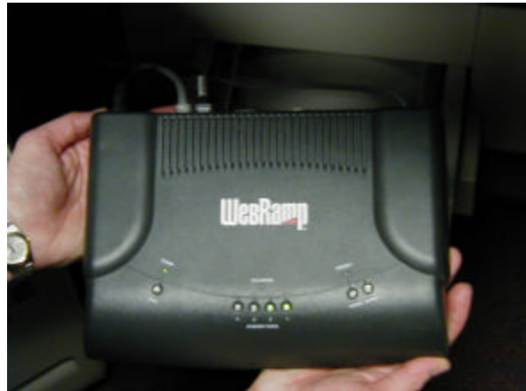
In order to speed up the communications network, River Valley Transit added an integrated Modem/Router to extend their LAN.
