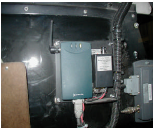
The RF Communications Units allow messages to be transferred between the MDTs and the Base computer.
