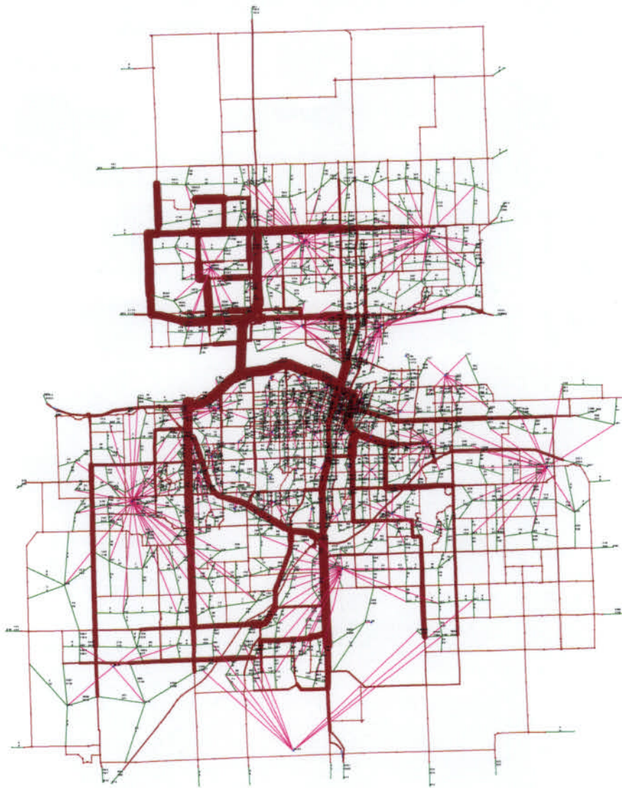
Figure C.1. Traffic assignment results due to activity allocation estimated by QRS II model
