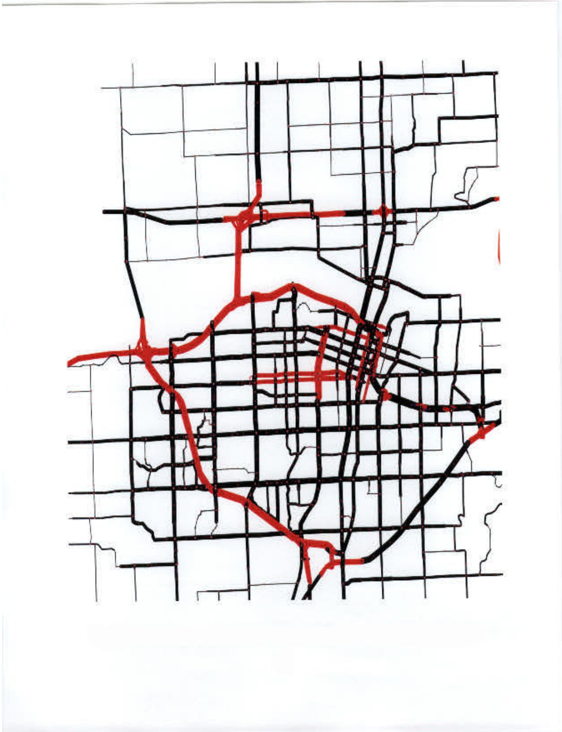
FIGURE A-1: Traffic Assignment Results on "NET 74R" Loaded with Census Data as Input
