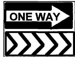
Figure 15. One Way and chevron sign combination for use in central island of roundabout.
