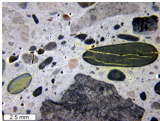
Figure 4. Stereo micrograph showing fine aggregate particles fractured due to ASR. Sodium cobaltinitrite was used to stain the ASR gel yellow, making it readily visible in the affected aggregate particles, cracks, and in the cement paste. (source: Karl Peterson)
