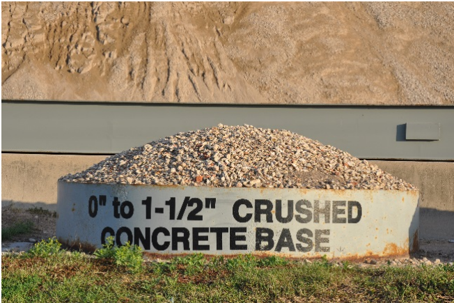
Figure 9. Photo. Reclaimed concrete crushed to be used as a base for concrete pavements.
