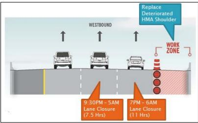
Figure 8. Illustration. Stage 1 lane closure and traffic flow.
