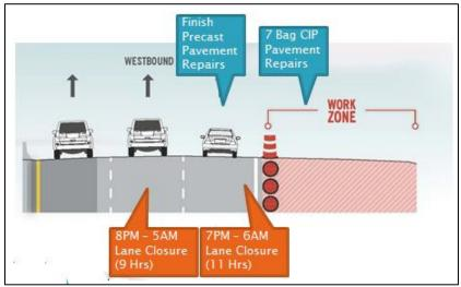
Figure 12. Illustration. Stage 3 outside shoulder and Lane 3 closure and traffic flow.
