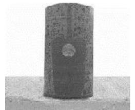
Figure 6. Photo. Bottom slot filled with grout.
