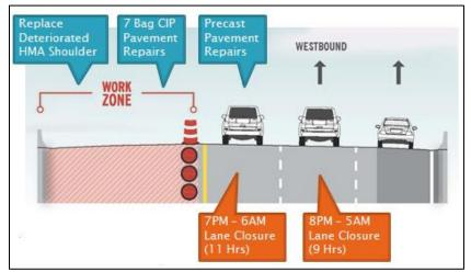
Figure 10. Illustration. Stage 2 lane closure and traffic flow.
