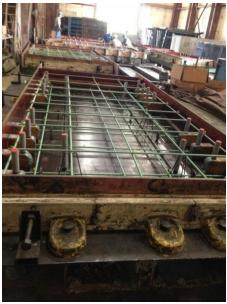
Figure 14. Photo. Panel setup.
