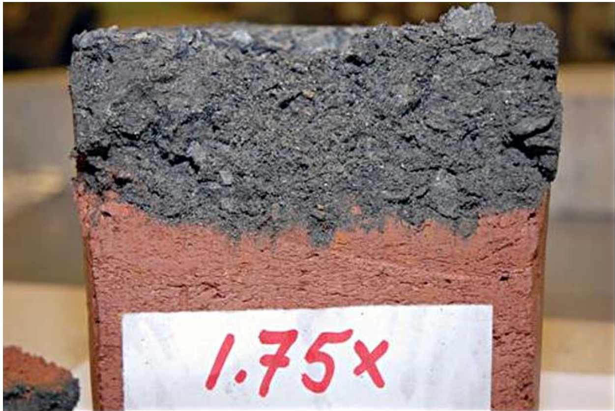
Figure 11. Cross Section of Sample without Geotextile: CBR 1.75 Soil and VDOT 21-B Aggregate
