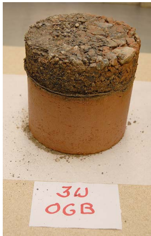
Figure 16. Slipping of Geotextile in Open-Graded Base Laboratory Sample
