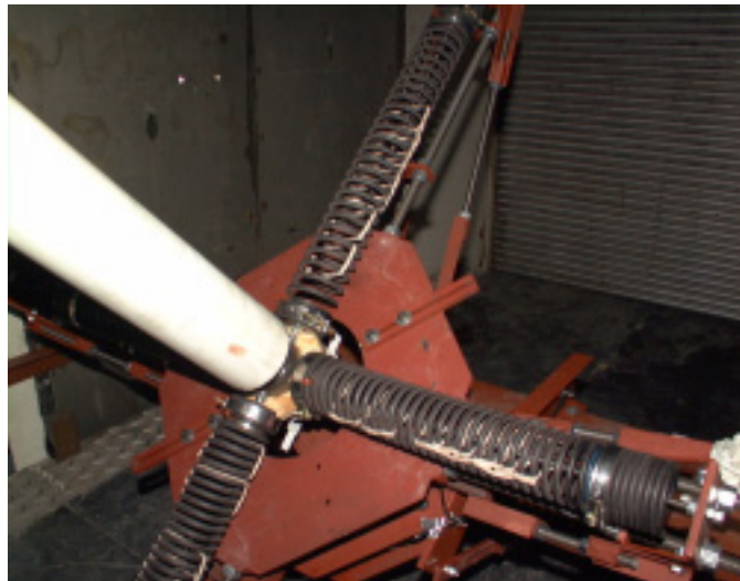
Figure 44: Elastic bands on the spring coils.
