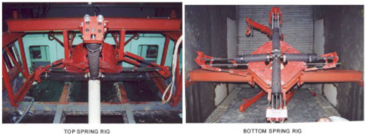
Figure 38: Cable supporting rig.
