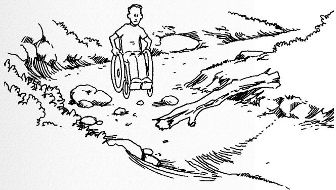
Figure 15-8. The tread obstacles on this trail surface do not allow this hiker to continue travel on the trail. Even when obstacles are avoidable, maneuvering around them requires trail users to expend more energy and time.
