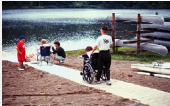
Figure 17-7. GOOD DESIGN: This temporary beach access route crosses the surface of the beach and extends to the high tide level.
