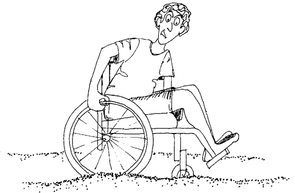
Figure 5-7: Soft surfaces are difficult for people with mobility impairments to negotiate and therefore should be avoided.
