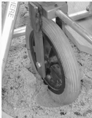
Figure 15-5. This rotational penetrometer is testing the firmness and stability of sand.
