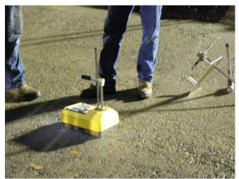
Figure 15. Photo. Base compaction testing using a nuclear gage.
