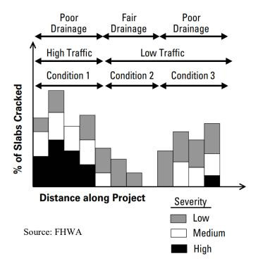
Figure 2. Example condition profile illustrating distress levels in an existing pavement (Smith et al. 2014).
