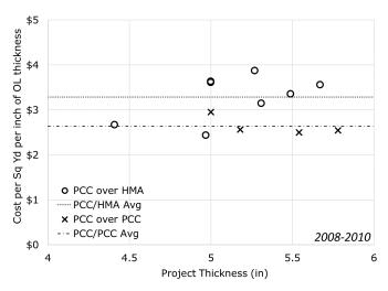
Figure 5. Overlay cost per square yard-inch of overlay thickness for twelve thin concrete overlay projects constructed in 2008 and 2009 in four states (data source: Fick 2010).
