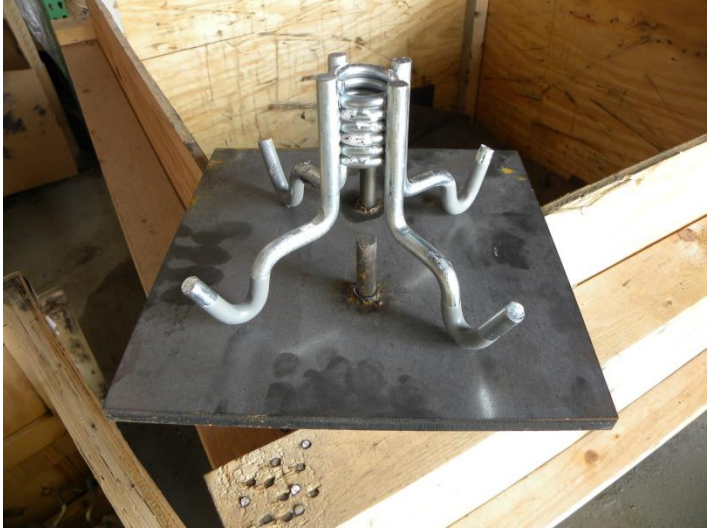
Figure 5. Photo. The leveling lift system – base plate and Dayton Superior Insert.
