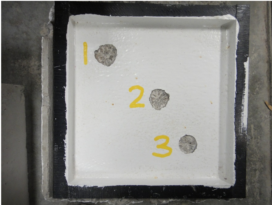
Figure 8. Salt ponding block after powder samples of concrete have been extracted after completion of the salt ponding test
