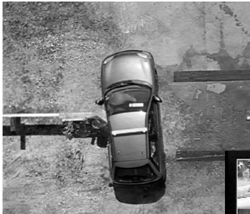
The modified ET-2000 guardrail end treatment performed well under a 35 mph side impact crash test.
