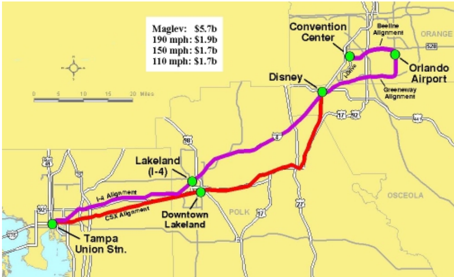
Figure 3.7: Route Alternative 6- Same as Alternative 5, but with the addition of an extension to Orange County Convention Center.
