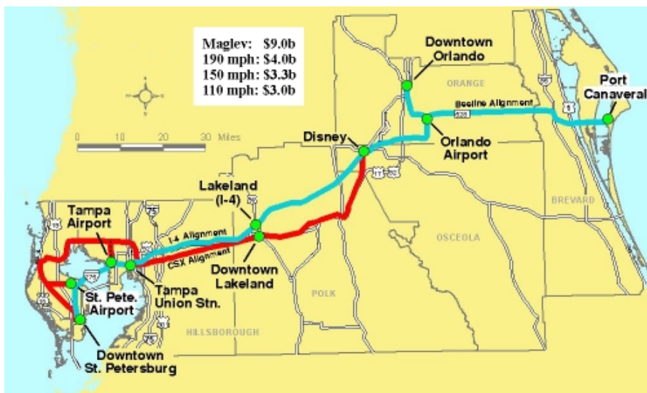
Figure 3.4: Route Alternative 3 - Connection from Downtown St. Petersburg to Port Canaveral using Greenway option through Orlando. Includes connection to downtown Orlando, however, there is no connection to Orange County Convention Center.
