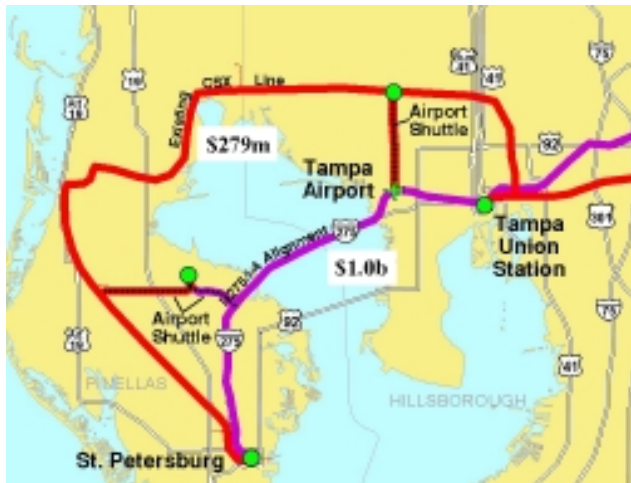
Figure 3.11: St. Petersburg-Tampa Segment Capital Costs. In the Tampa-St. Petersburg region, there are two alternate alignments that could serve the areas destinations. The costs include only infrastructure costs for building non-electrified 150mph technology.
