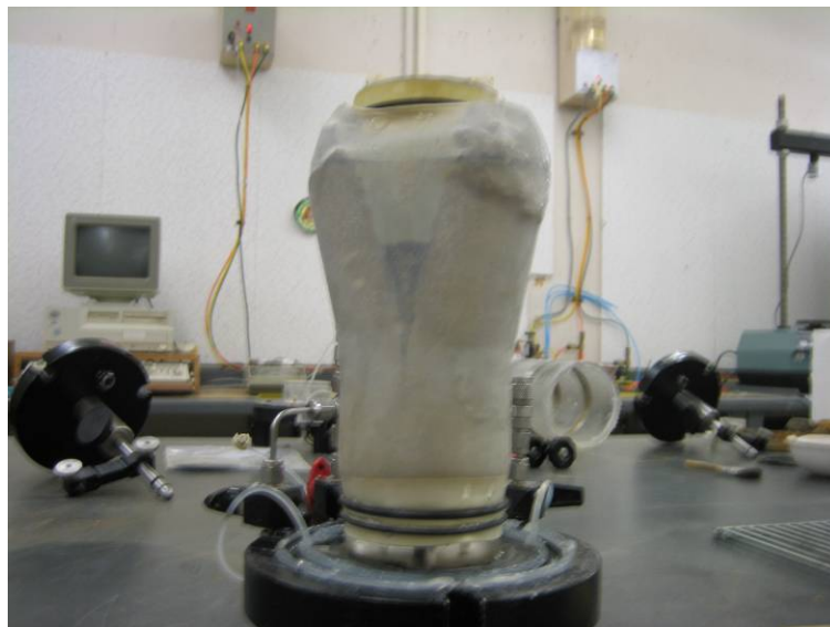
Figure 4.30: Splitting type of failure for 10% cement treated Aberdeen soil.
