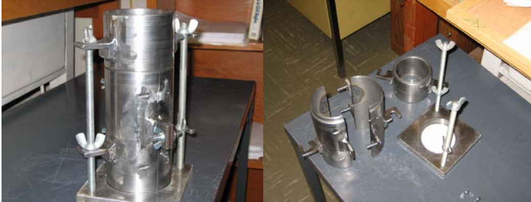
Figure 3.8: Custom built mold for triaxial test.
