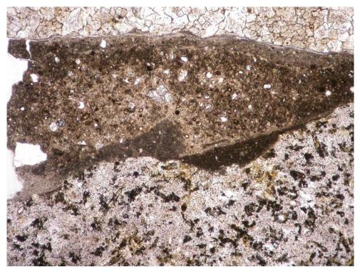
Photo #6: Thin section photomicrograph of paste inhomogeneities in Sample #2. Planed-polarized light; Field Length = 2.8 mm
