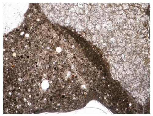
Photo #5: Thin section photomicrograph of paste inhomogeneities in Sample #1. Planed-polarized light; Field Length = 2.8 mm
