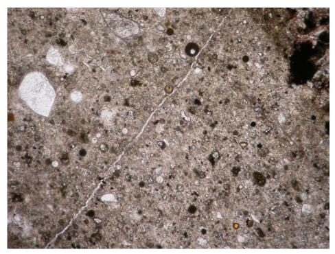
Photo #3: Thin section photomicrograph of the paste in Sample #3. Plane-polarized light; Field Length = 1.4 mm
