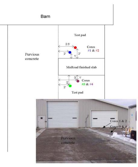
FIGURE B-1: Schematic and photo showing the layout of the pervious concrete at MnRoad. Cell-64 Pervious Concrete Driveway is in foreground, test pads are to the far right (schematic is not to scale).
