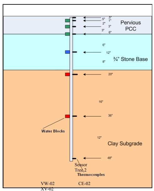
FIGURE 3: Cell 64 sensor tree (profile view, not to scale).
