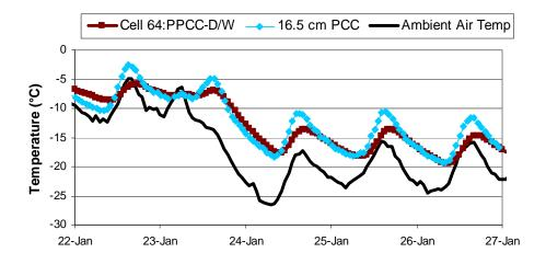
FIGURE 14: Mid-depth temperature in pervious (PPCC) and impervious (PCC) test cells at MnROAD.
