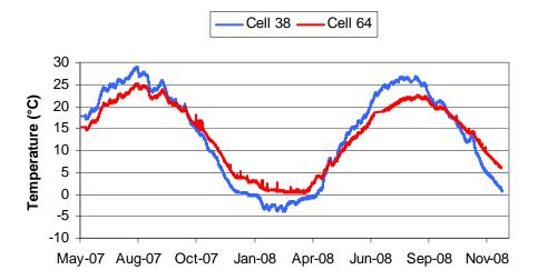
FIGURE 13: Temperature 36 in. below pavement surface.
