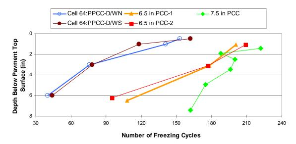
FIGURE 12: Number of freezing cycles at various depths below pervious and impervious PCC pavements of similar thickness.
