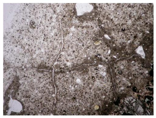
Photo #9: Thin section photomicrograph of the extensive cracking in Sample #1. Plane-polarized light; Field Length = 2.8 mm
