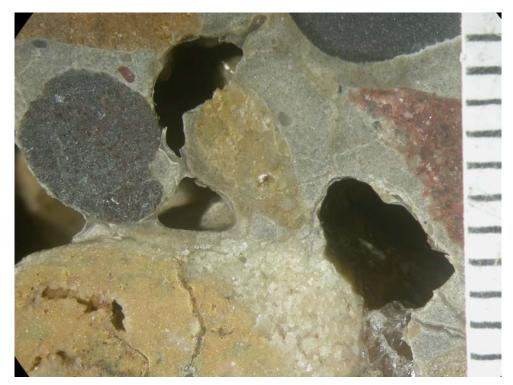
Photo #12: Photomicrograph of the air voids in Sample #2. Note the lack of entrained air in the paste regions. Scale: 1 division = 1 mm
