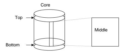
FIGURE B-2: Illustration of how cores are sectioned for microscopic evaluation.
