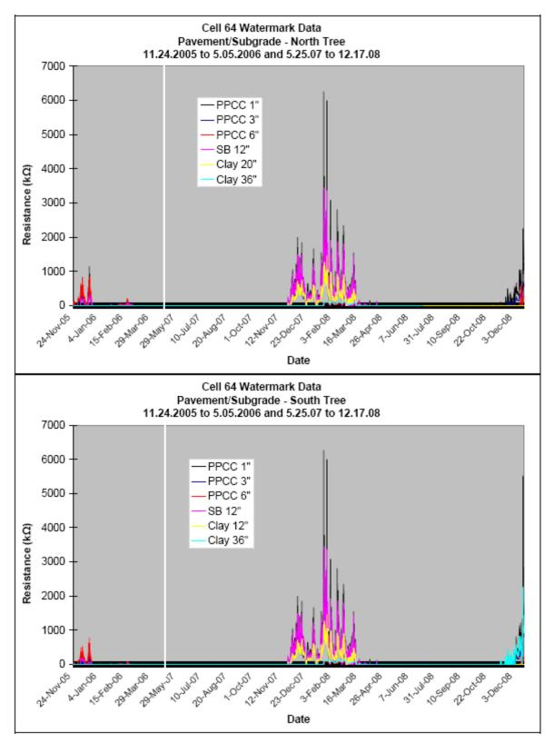
FIGURE 10: Freeze-thaw cycles measured by watermarks in pavement, base, and subgrade.
