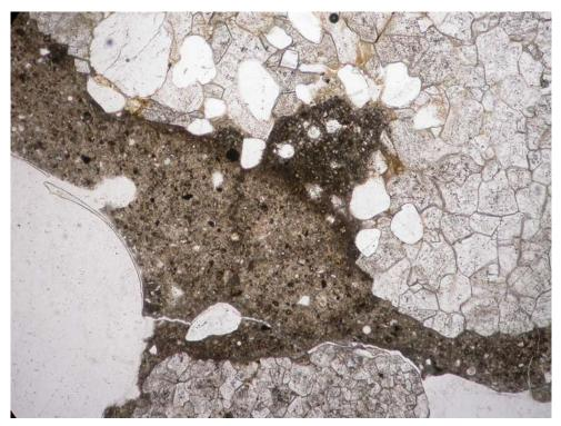
Photo #7: Thin section photomicrograph of paste inhomogeneities in Sample #3. Planed-polarized light; Field Length = 2.8 mm
