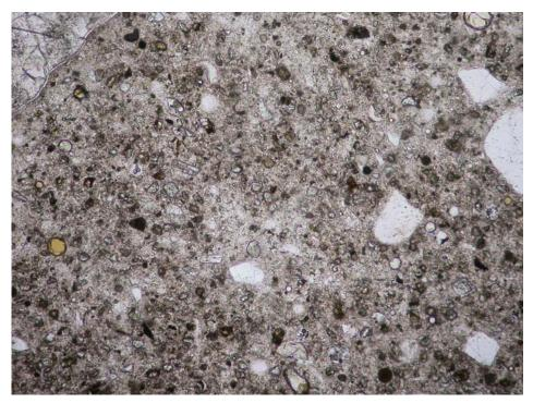
Photo #1: Thin section photomicrograph of the paste in Sample #1. Plane-polarized light; Field Length = 1.4 mm
