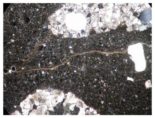
Photo #10: Thin section photomicrograph of a microcrack that has autogenously healed. Cross-polarized light; Field Length = 2.8 mm
