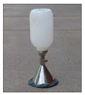
FIGURE 7: In-situ drainability measurement device.
