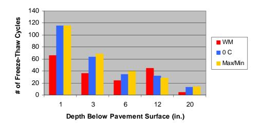
FIGURE 11: Comparison of number of freeze-thaw cycles calculated using different definitions at various depths below Cell 64.
