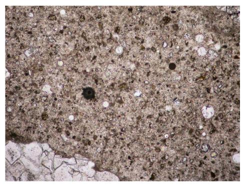
Photo #4: Thin section photomicrograph of the paste in Sample #4. Plane-polarized light; Field Length = 1.4 mm
