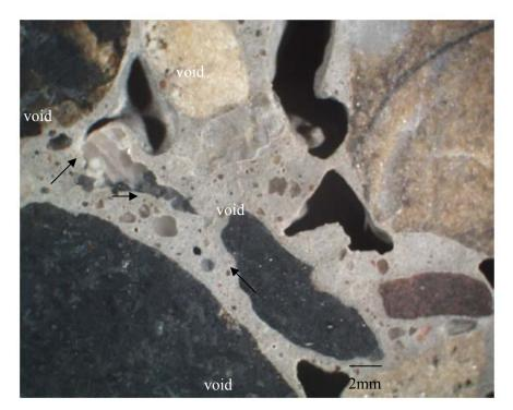
FIGURE B-3: Arrows point to fine cracks in paste in core 2.
