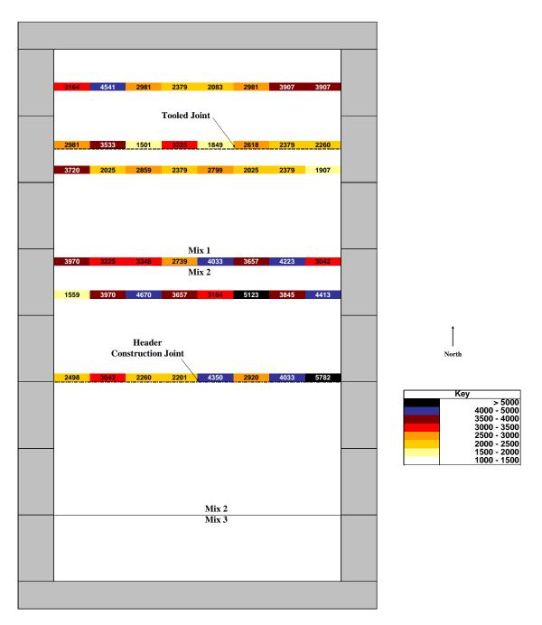
FIGURE 6: Schmidt hammer measurements on April 2, 2009.
