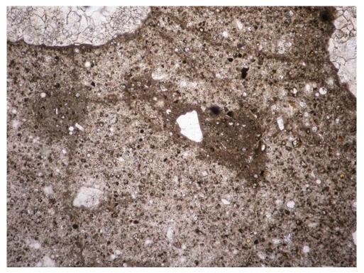
Photo #8: Thin section photomicrograph of paste inhomogeneities in Sample #4. Planed-polarized light; Field Length = 2.8 mm
