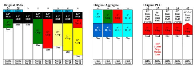
FIGURE A-3: MnROAD Phase I Low Volume Road (LVR) test sections.
