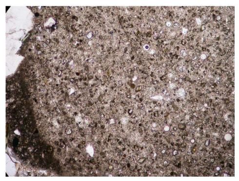
Photo #2: Thin section photomicrograph of the paste in Sample #2. Plane-polarized light; Field Length = 1.4 mm
