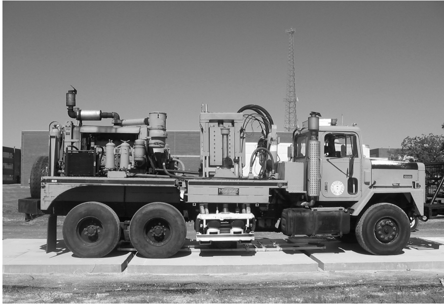
(a) SDD positioned over testing slab
