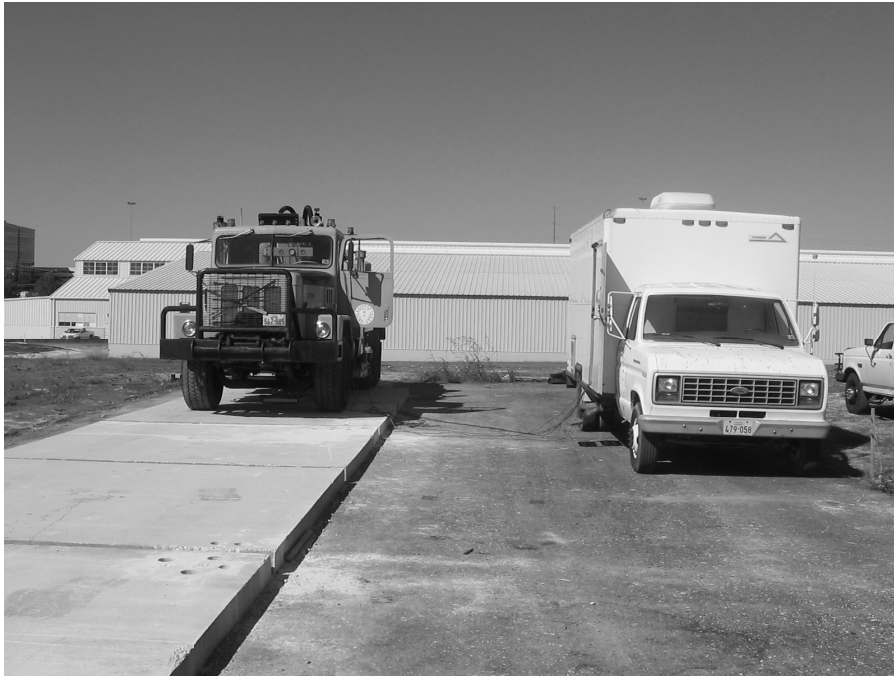
(b) Super-accelerated fatigue testing system using SDD
