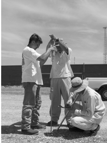
(a) Dynamic cone penetration (DCP) testing on subgrade
