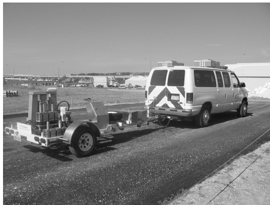
(c) Falling weight deflection (FWD) testing on asphalt stabilized base
