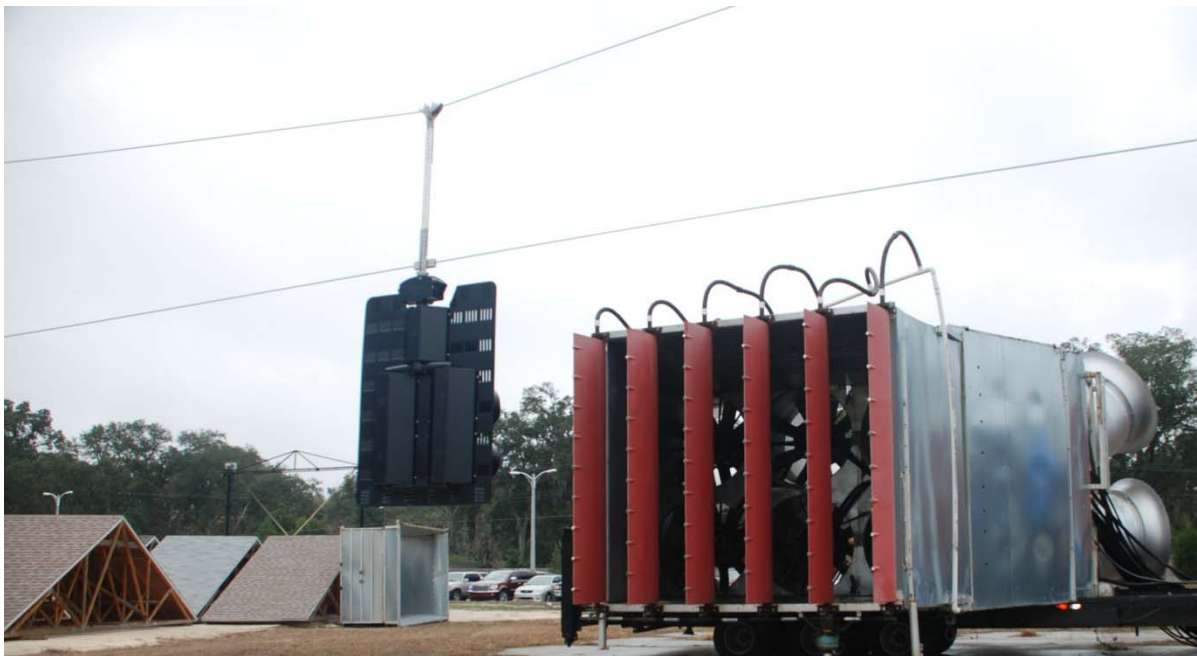
Figure 3-4. The UF Hurricane Simulator's fans and wind vanes (front) (Photo courtesy of author)
