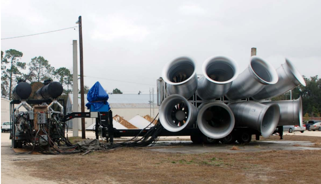
Figure 3-3. The UF Hurricane Simulator's engines and fans (back) (Photo courtesy of author)
