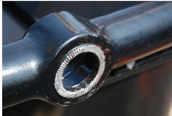
Figure 6-2. Worn serrated teeth on two-way bracket which connects to top signal head (Test 22) (Photo courtesy of author)
