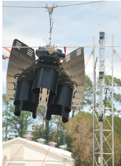
Figure 3-10. Mounting system for string potentiometers (Photos courtesy of author)
