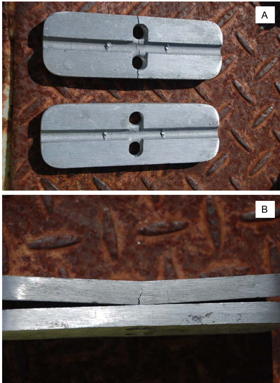
Figure 6-5. Failed sand cast aluminum stabilizer clamp: A) parts shown lain separated; B) parts shown together (Photos courtesy of author)
