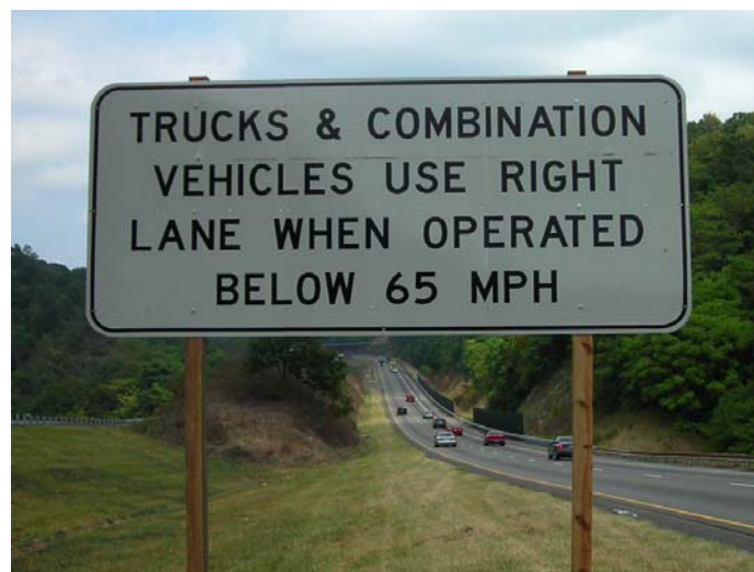
Figure 2. 2007 Truck Restriction Sign Used on Interstates with Two Directional Lanes and Steep Grades
