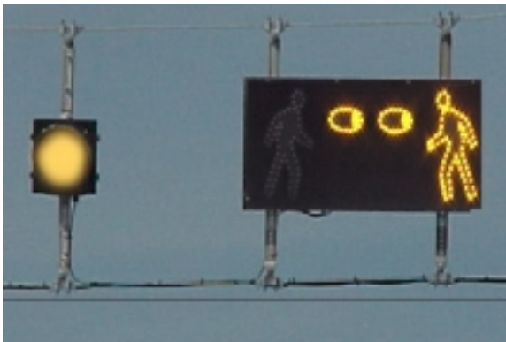
Overhead signals to warn drivers of the presence of pedestrians in an approaching crosswalk.
