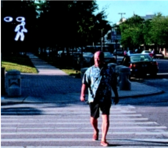
A pedestrian crosses at a crosswalk equipped with scanning eye pedestrian heads.
