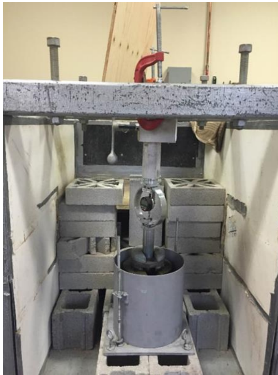
Figure 54: Testing setup for large-scale CBR tests.
