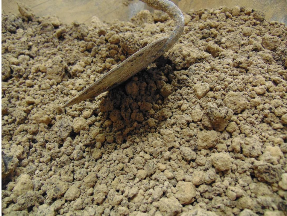
Figure 48: Close-up of soil mixed with 12% fly ash.
