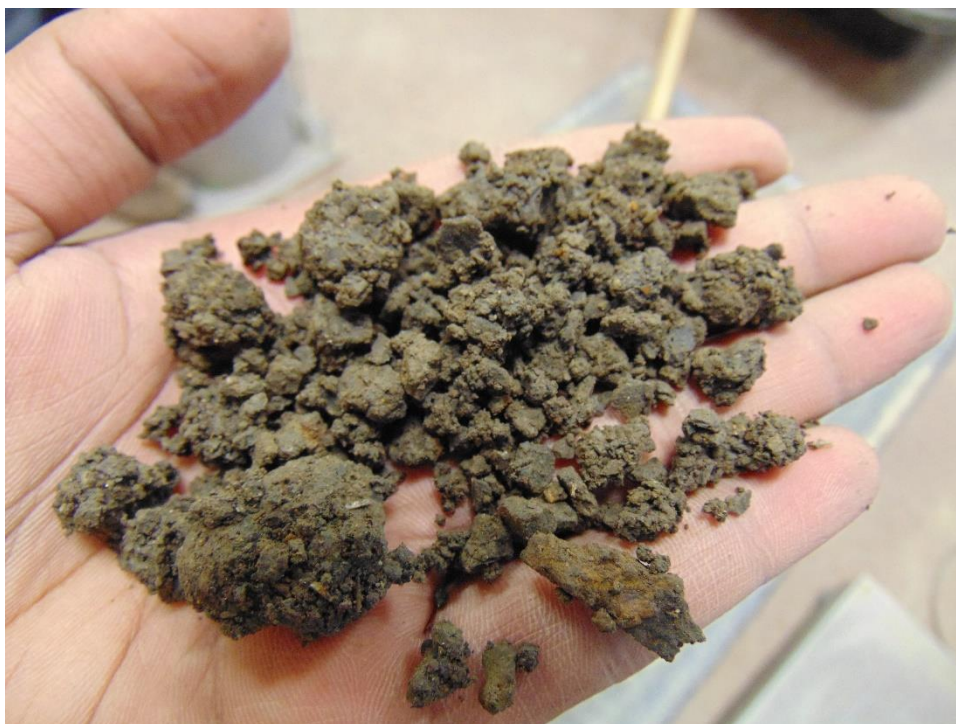
Figure 46: Typical particle sizes after the moisture conditioning process.
