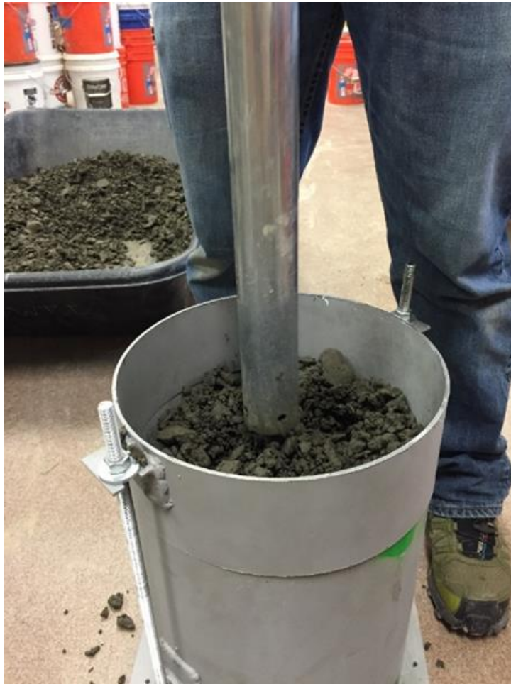
Figure 49: Compaction of soil into large-scale CBR molds.
