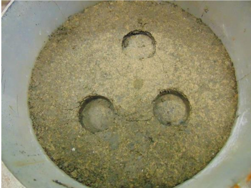
Figure 53: Photograph of the soil surface after CBR testing large-scale sample.
