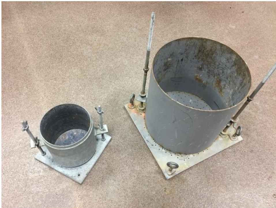
Figure 45: Photo of standard 6-in. CBR mold compared to the large-scale 12-in. CBR mold.
