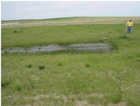
Figure 28: Site 3, soil sample location on east side of fault (heave) showing standing water on west side of fault.
