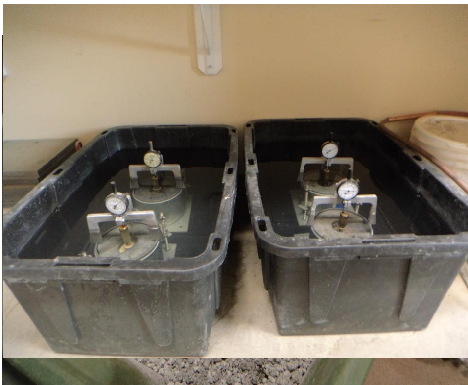
Figure 44: Compacted CBR soil samples in soaking tank.
