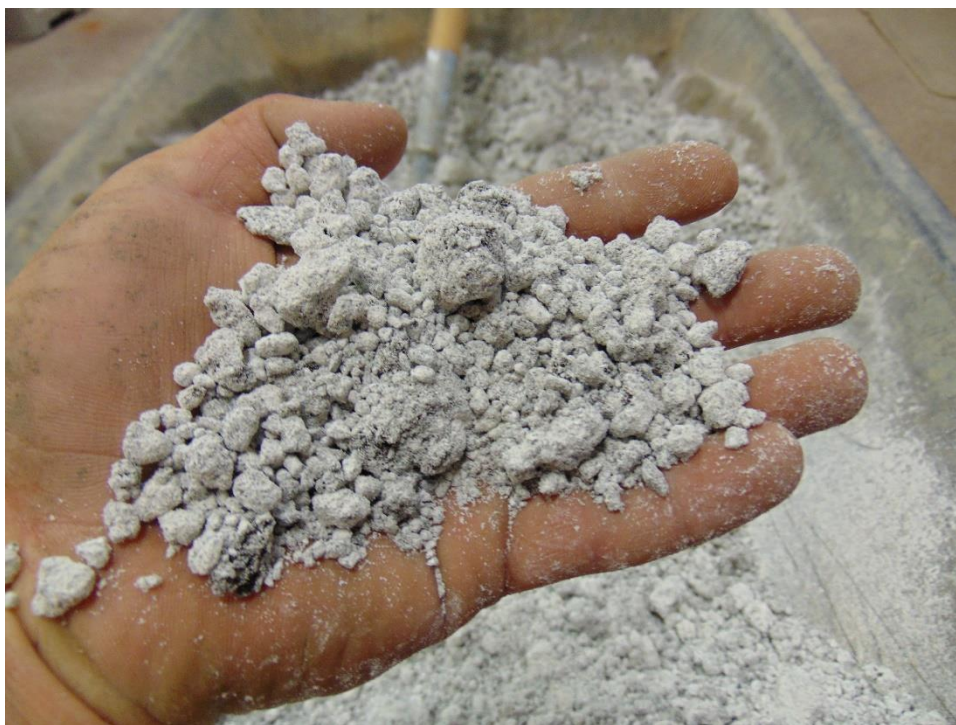
Figure 47: Close-up of soil mixed with 9% lime.
