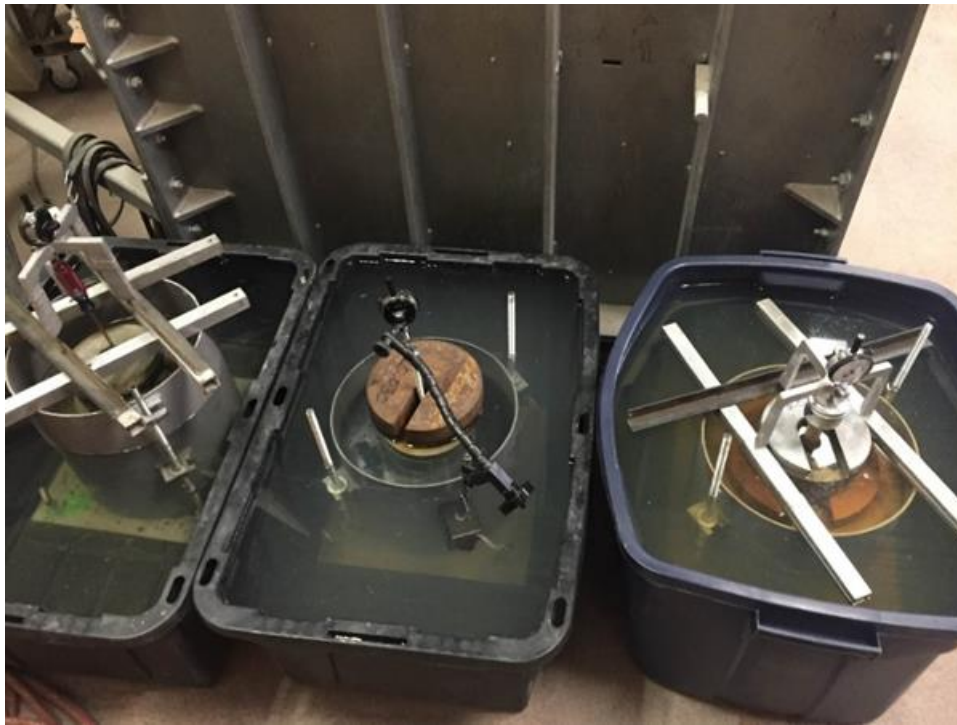
Figure 51: Setup for large-scale CBR tests during the 96-hour soak period.
