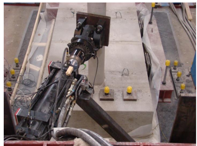
(b) Actuator Set Up (15° Out-of-Plane)
