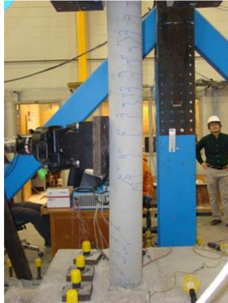
(b) Cracking in the Loaded Column
