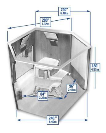
Figure 1. Schematic illustration of the Mark II motion-based simulator
