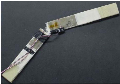
(c) Tension Coupon of Core Laminate
