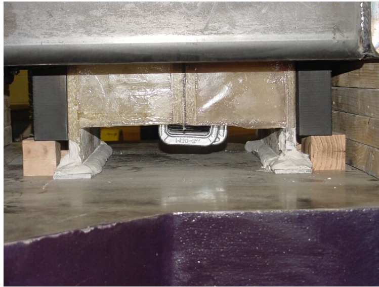
Figure 3.18: Detail of the Bottom Portion of Confined Double-Shear Specimen, Steel Plates are Supported on Wooden Blocks (Photo)
