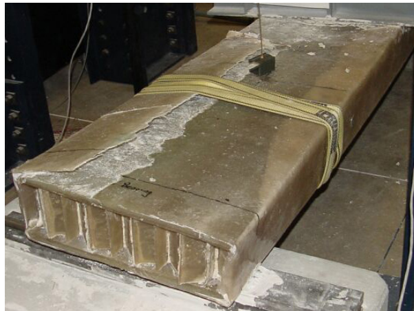
(c) Specimen A18 Repaired (Horizontal Shear Failure Resulted in Wrap Delamination)
