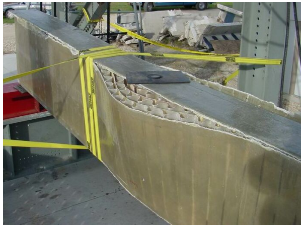
(b) 32-ft-long Repaired Beam
