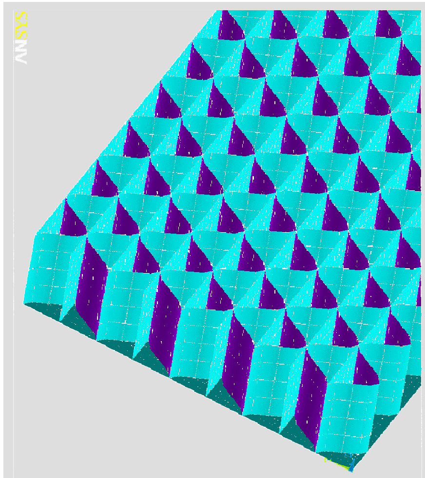
Figure 4.12: FRPH Panel Mesh in ANSYS Generated by MeshIt
