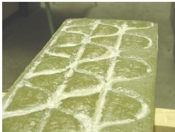
Figure 4.7: Photos Showing Deformations in the Face Laminate of a FRPH panel
