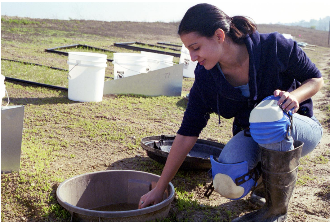
Figure 6.2. Collecting water and sediment from field erosion experiment.
