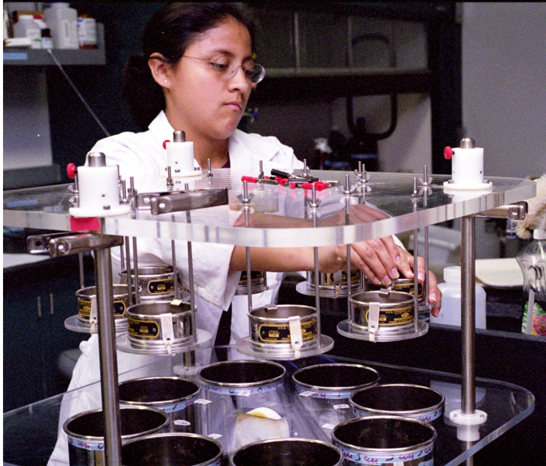
Figure 4.1. Soil samples loaded onto to wet sieving apparatus are assessed for their stability in water.
