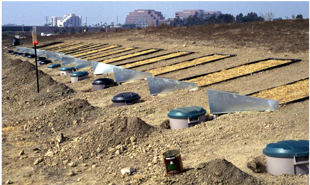
Figure 6.1. Field erosion demonstration experiment using 20 plots inoculated with mycorrhizal fungi.
