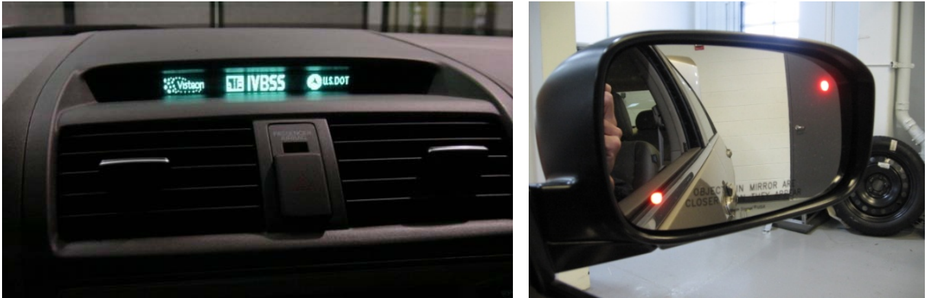
Figure 17. Visual display (left) and blind spot detection icons installed in the Honda Accord
