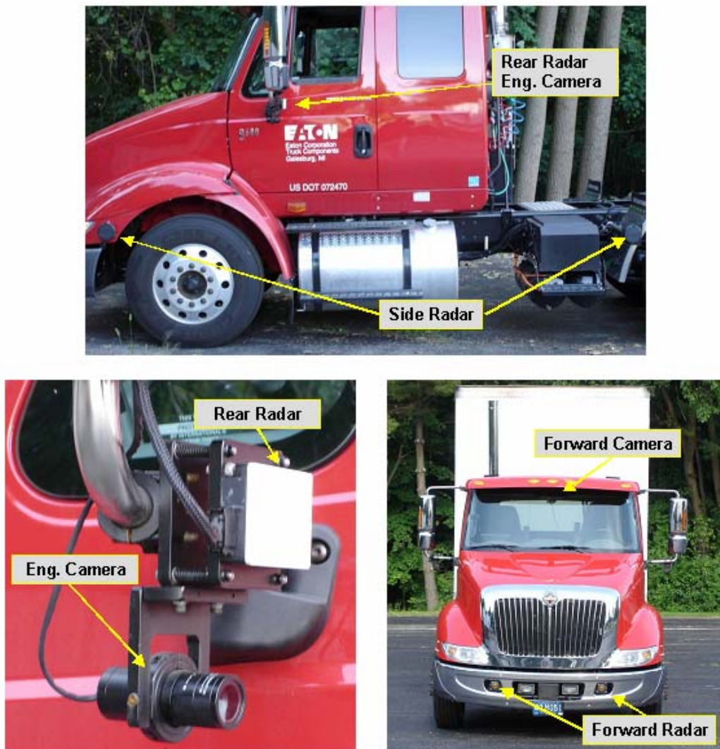
Figure 32. Bronze tractor sensor mounting
