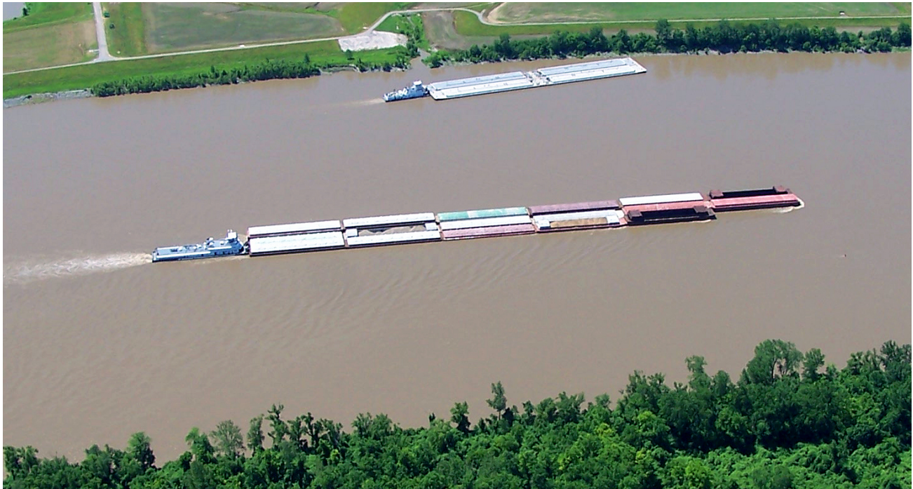
Figure 13, Illustration of Two Tows on the Mississippi River. The bigger tow has 17 barges, only 2 more than normal for a "standard tow" of 15 barges.
