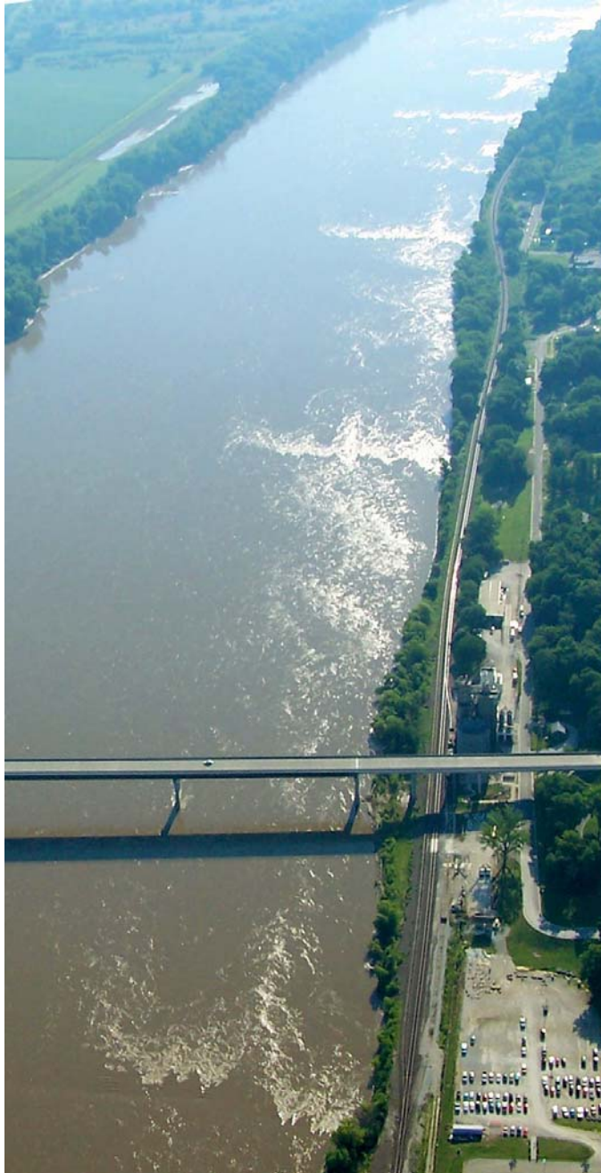
Figure 26, The Missouri River at Boonville with Regular Surface Disturbances Caused by Wing Dikes.
