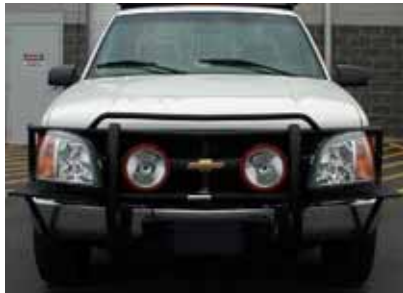
Figure 7. Photo. Pickup with HOH and HHB.
