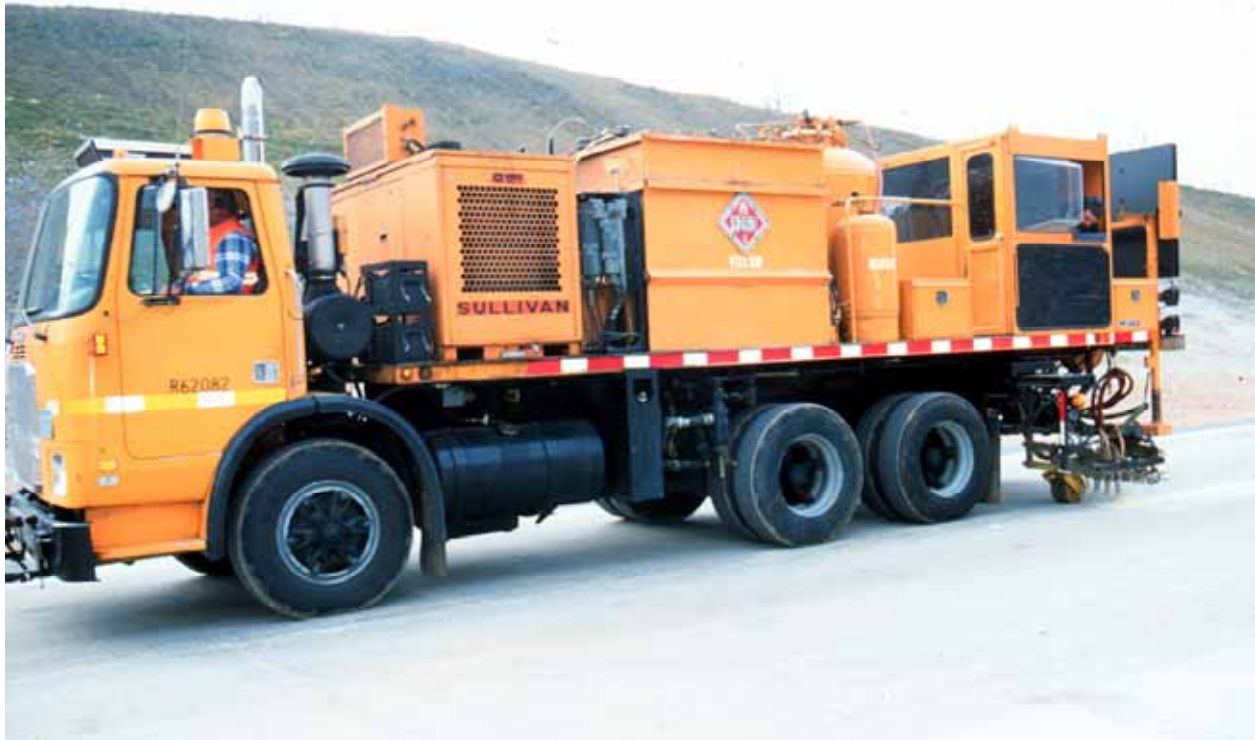
Figure 4. Photo. Application of the fluorescent pavement markings using the long-line truck.
