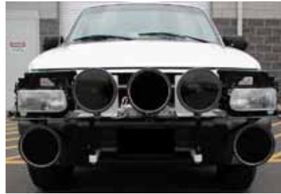
Figure 6. Photo. SUV 2 with three or five UV-A and HLB or HID.
