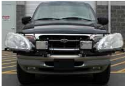
Figure 5. Photo. SUV 1 with hybrid UV-A + HID.
