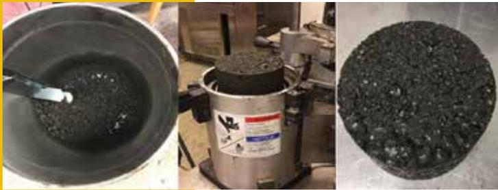
© 2017 Department of Civil and Environmental Engineering, Washington State University. Researchers created a rotary reactor to simulate the production of the hot-mix bio-binder through mixing aggregates with bio-asphalt.
