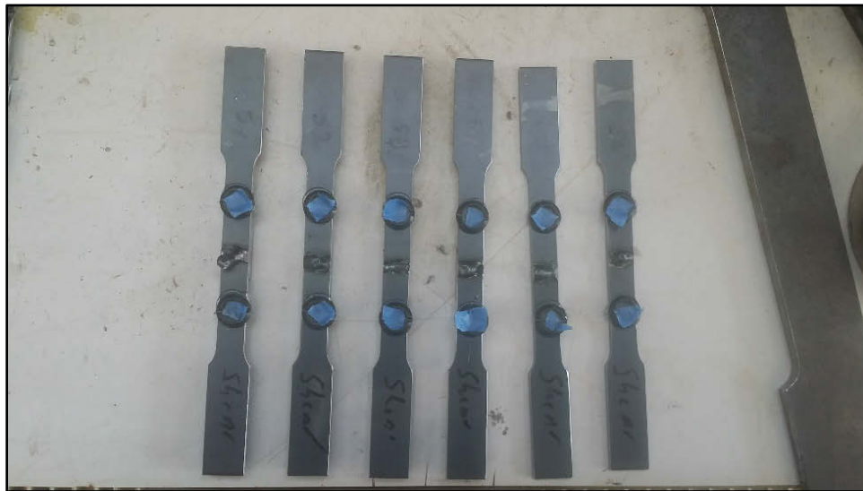
Figure 3.37: Welded test coupons for cutting method comparison.
