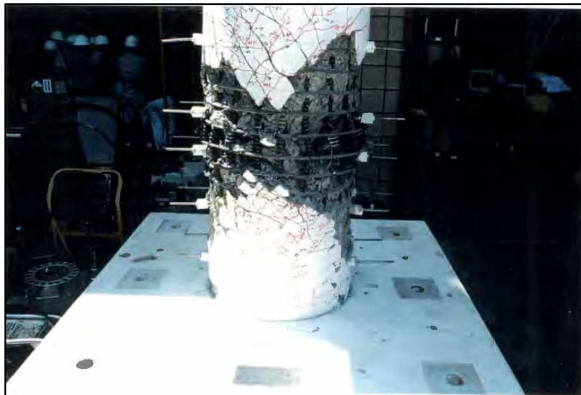
Figure 1.5: Relocated plastic hinge in RC bridge column by (Hose et al., 1997) at USCD laboratory.
