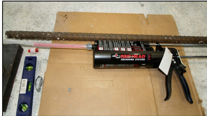
Figure 3.17: Redhead two-part epoxy application system.
