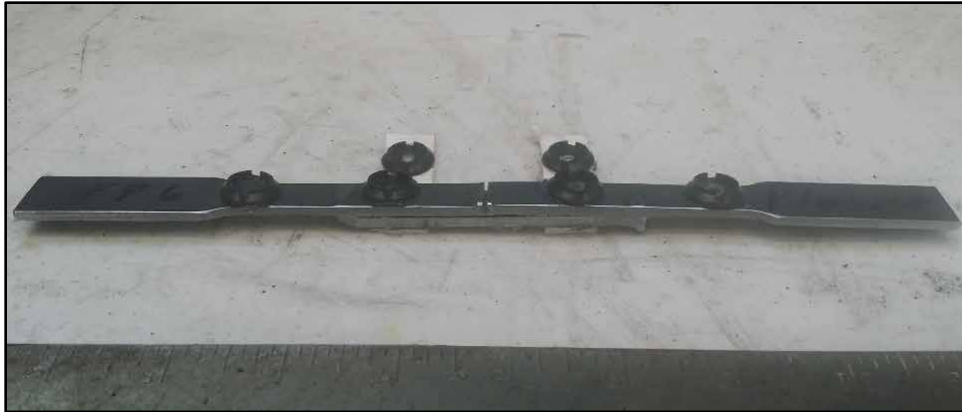
Figure 3.41: Welded coupon with patch repair.
