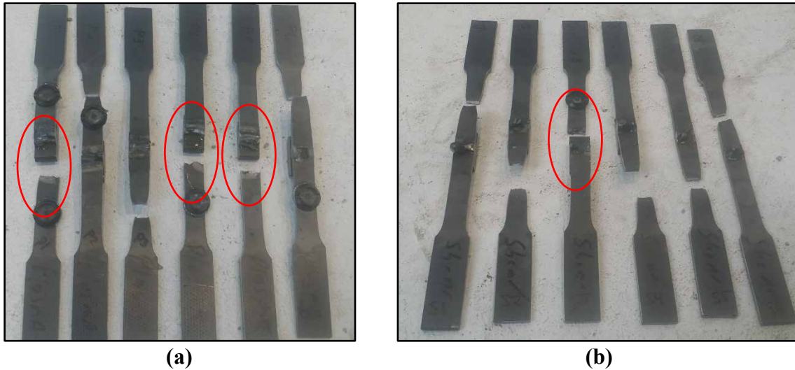
Figure 3.39: Tested samples constructed using a welded edge cut by (a) plasma torch; and (b) shear cut.
