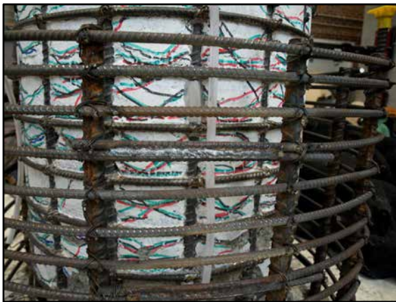
Figure 3.31: (a) Repair #4 rebar hoop splice weld; (b) Repair #4 splice weld detail.
