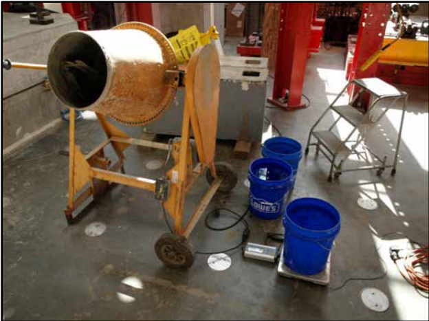
Figure 3.25: Electric drum mixer and grout mixing station.
