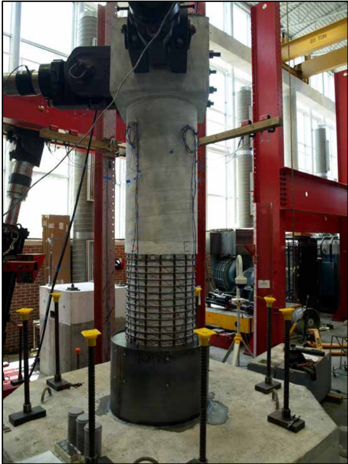
Figure 3.28: Completed repair installation on lab specimen.
