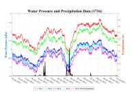
The pore water pressure in the backfill was maintained at low levels with both drainage systems. (Left: with PCDS; Right: with Porous Backfill)
