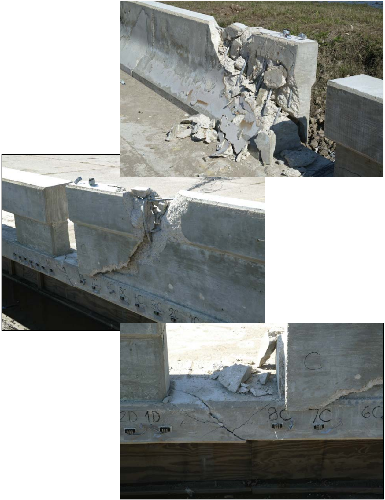
Figure 19. Bridge Rail T501 at Location C after Test B6.
