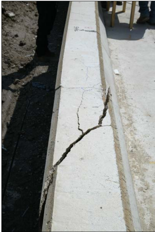
Figure 10. Bridge Rail T501 at Location B after Test S5.
