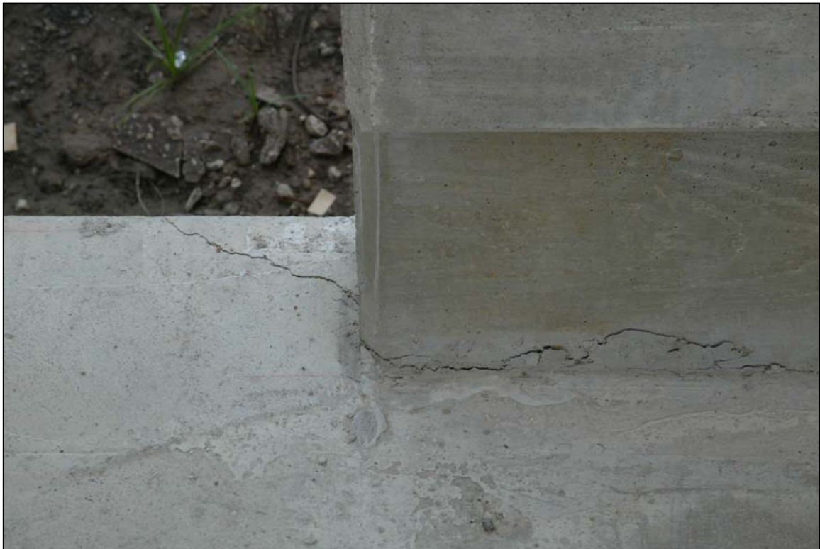
Figure 8. Bridge Rail T203 at Location D after Test S3.
