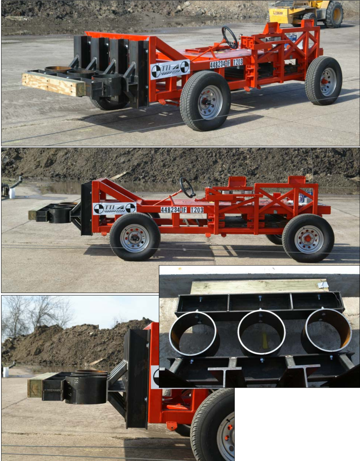
Figure 13. Bogie Vehicle Used in Dynamic Load Testing.
