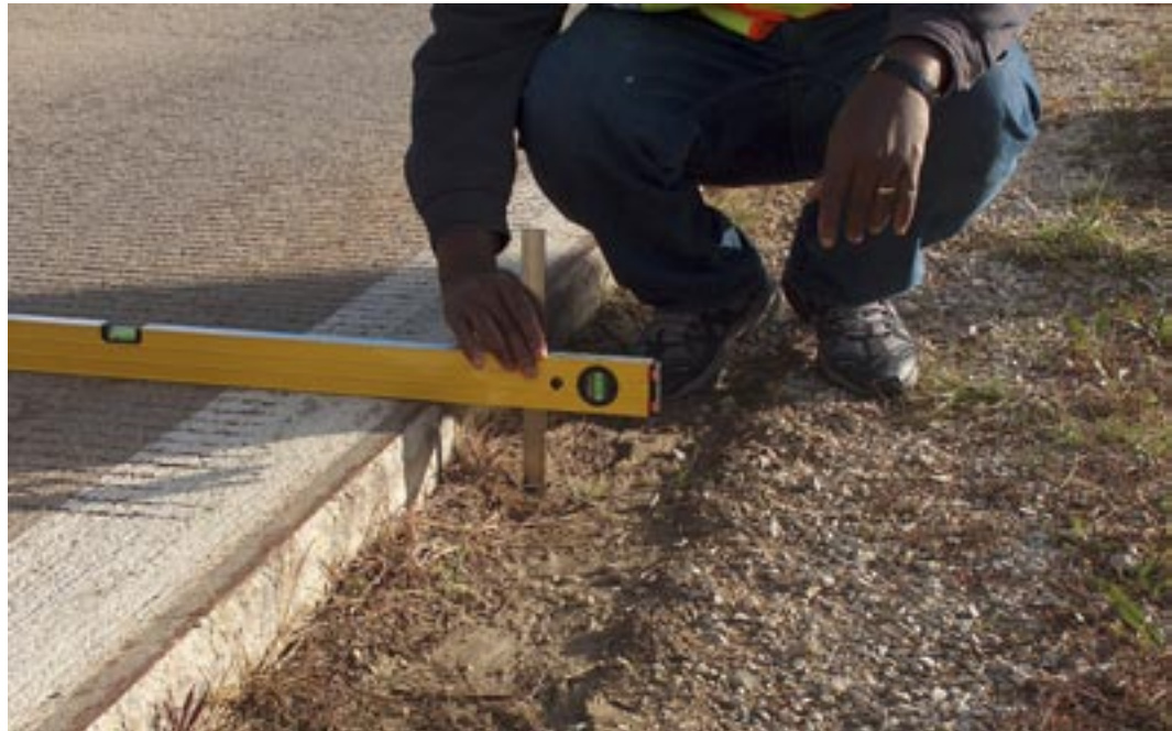
Figure 4-2. Measurement of edge drop-off height
