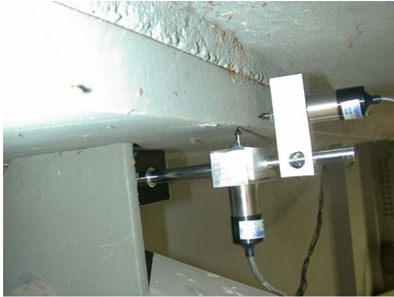
a. Photograph of out-of-plane and tipping transducers.
