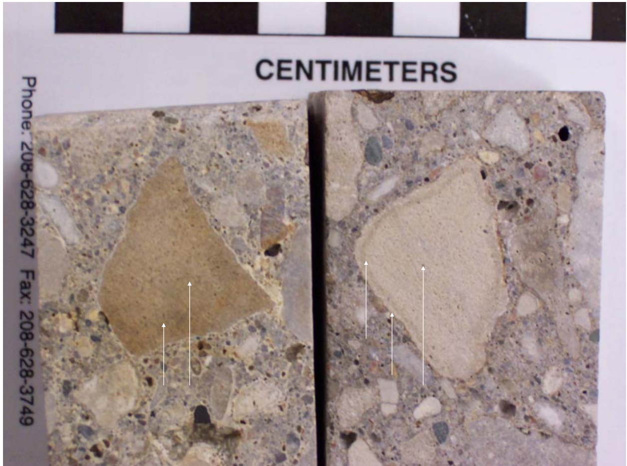
Figure 3. Concrete samples O5BB (left) and P3TB (right) showing compositional rims on dolomite particles that formed by dedolomitization reactions associated with the application of NaCl deicing salts.
