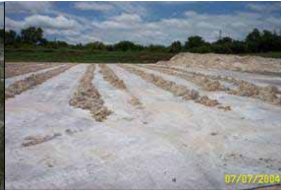
Figure 5: Solar drying of sludge in windrows
