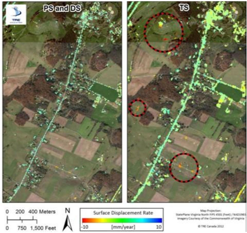
Figure 4 - Comparison between the PS and DS results (left) and the TS results (right). Note the subsidence areas identified on the right by the use of the TS technique.
