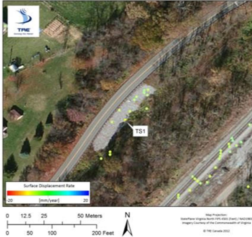
Figure 37 - InSAR points at the riprap slope along Greenville School Road.
