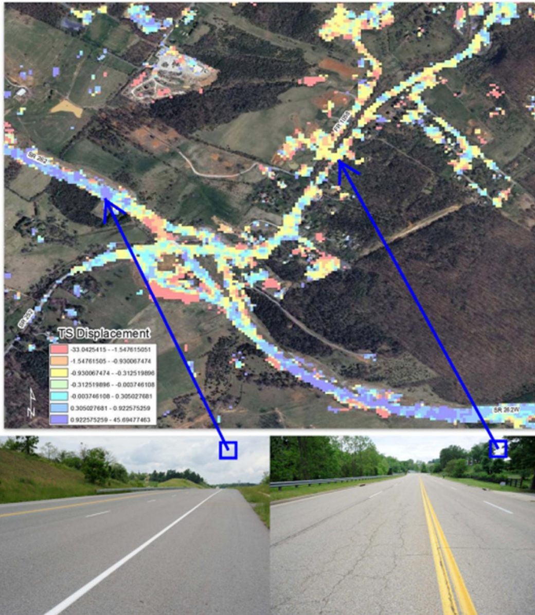
Figure 49 - TS results corresponding to pavement in good condition at Route 262 (bottom left) and one in poor condition at Middlebrook Avenue (bottom right).
