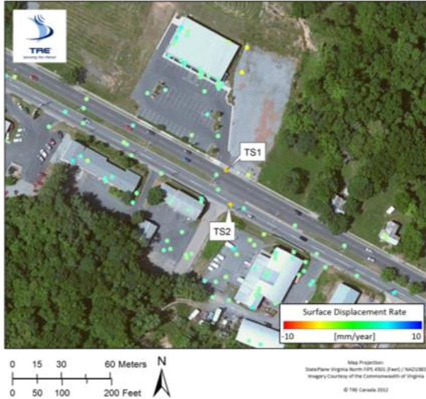
Figure 15 - A close-up of displacement results over a portion of the Virginia AOI designated as Area 4 in Figure 14.
