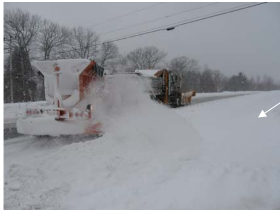
Photo 1: Clearing Travel Lane and Shoulder
