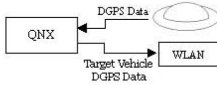
Figure 26 Overview of the system setup in the target vehicle
