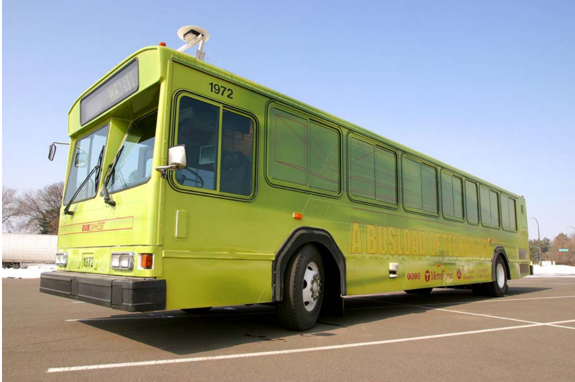
Picture 2. Research Vehicle “Technobus” as supplied by Metro Transit. The Technobus is equipped with a lane assist system for narrow lane guidance, and forward, left, and right side collision avoidance systems.
