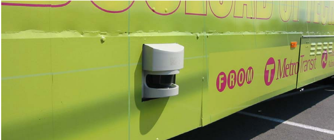
Picture 10. Scanning LIDAR sensor on left side of Technobus. Identical sensor is located on the right side of the bus. Image processing of left side sensor is optimized to detect vehicles adjacent to the bus; image processing of right side sensor is optimized to detect passengers entering and exiting the bus.
