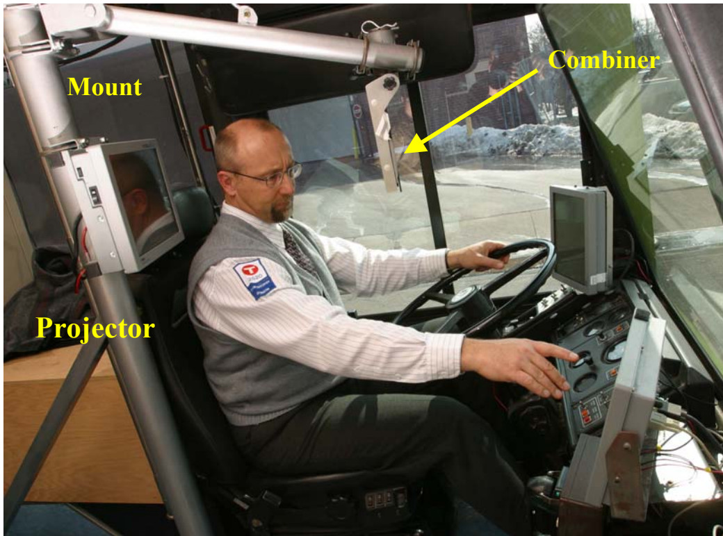
Picture 12. HUD System as it is mounted in the Technobus. Combiner and projector are mounted to a research grade (i.e., highly configurable) mechanical mount.
