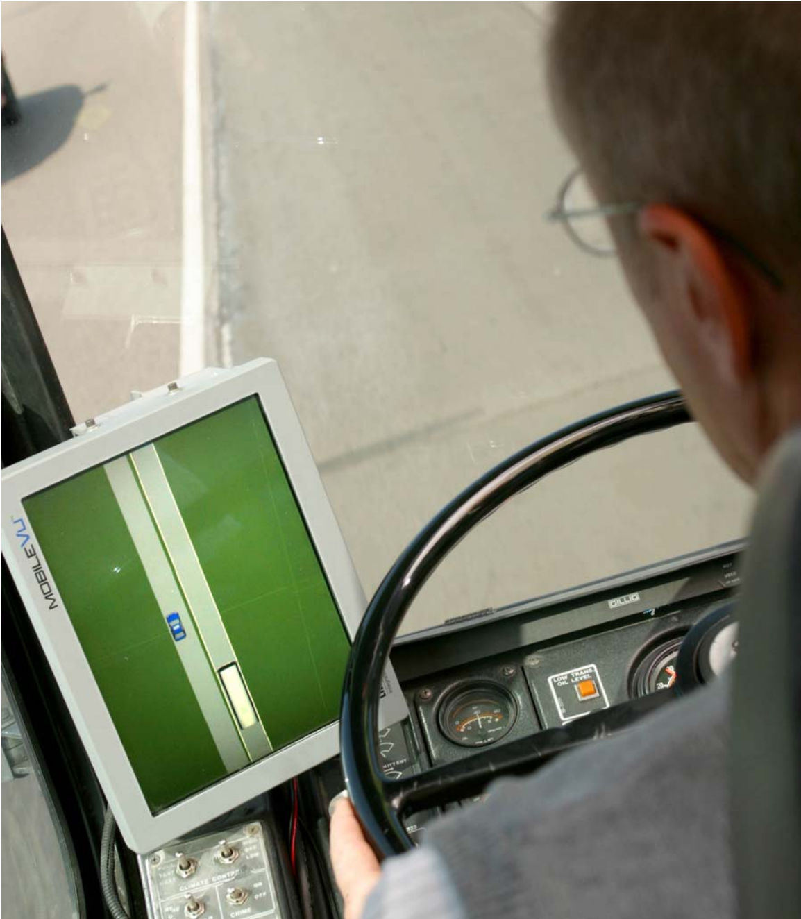
Picture 4. Picture of Virtual Mirror Display on the Technobus. In this plan view, the shoulder and adjacent lane of traffic are shown in grey, the top of the bus in white, and a radar or lidar detected obstacle in blue. The shoulder and lane information is provided by the on-board geospatial database.
