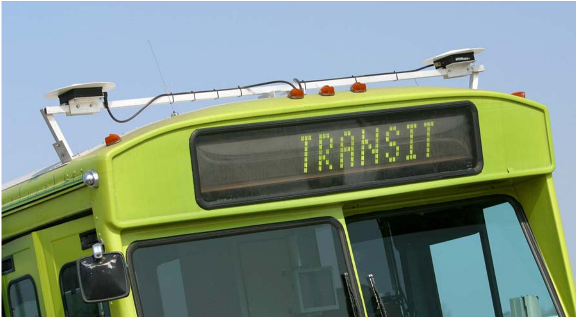
Picture 8. Front of Technobus showing GPS Antenna. Use of dual GPS receivers improves system robustness and provides vehicle position, heading, and roll measurements.
