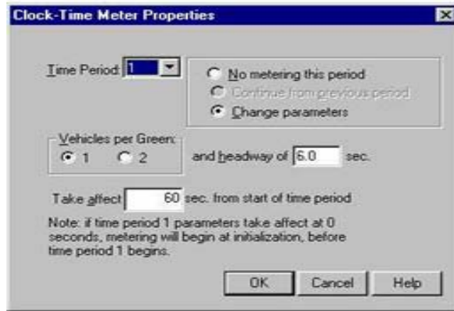
Figure 4-3: Clock- time meter properties (FHWA, 1996)
