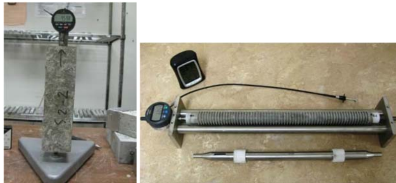
Figure 3.5: Drying shrinkage (left) and autogenous shrinkage (right)
