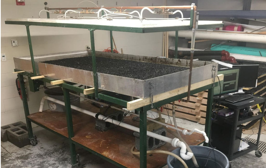
Figure 2: Testing a chip seal specimen in the rain simulator machine at Missouri S&T
