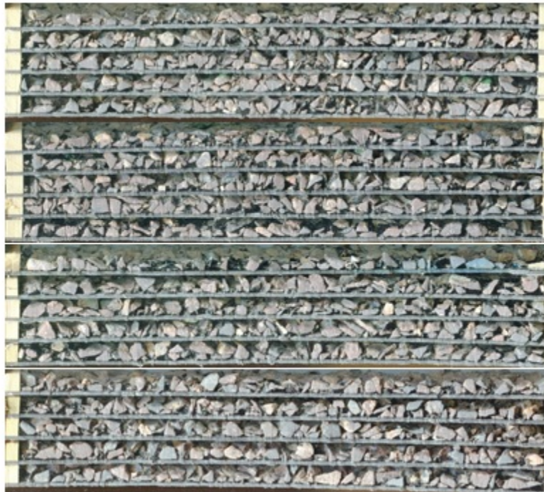
Figure 13: Chip seal sections for image processing for specimens with 100% trap rock aggregate
