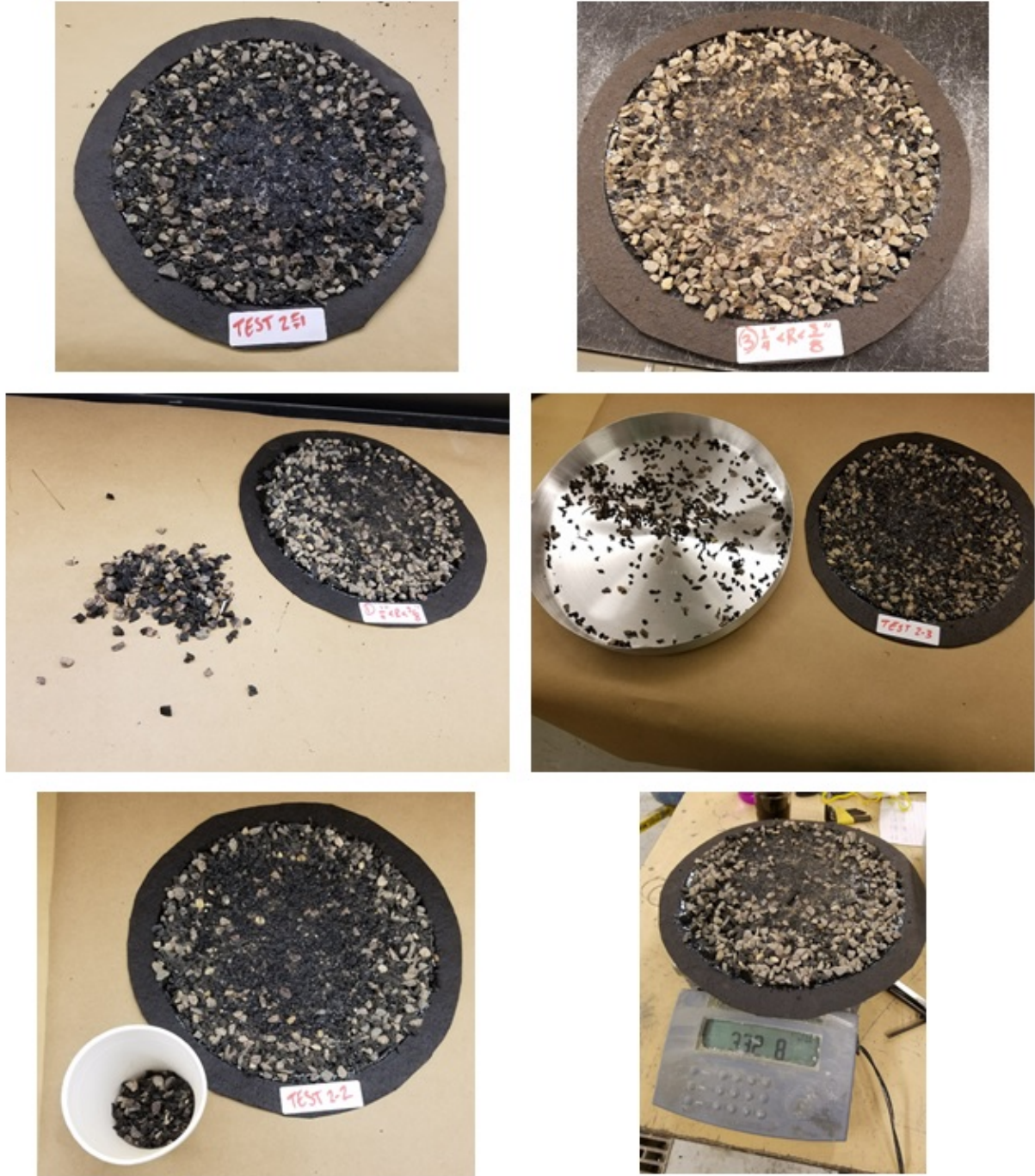
Figure C-6: Chip seal specimens with different rubber sizes after sweep test
