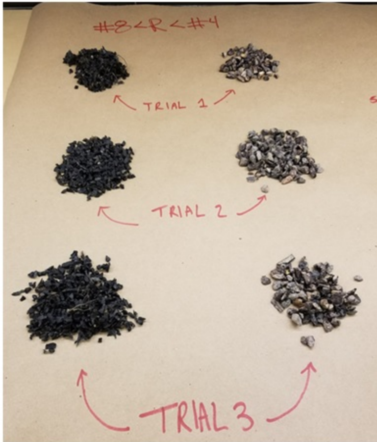
Figure C-5: Chip seal specimens with different rubber sizes during sweep test
