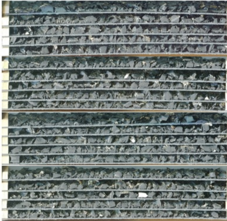
Figure 14: Chip seal sections for image processing for specimens with 100% rubber aggregate
