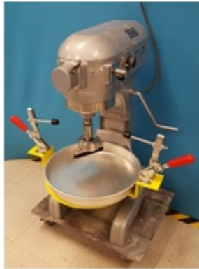
Figure C-2: Sweep test equipment (a) holding pan and brush holder, (b) specimen compactor (c) testing apparatus set-up, and (d) standard asphalt felt disks
