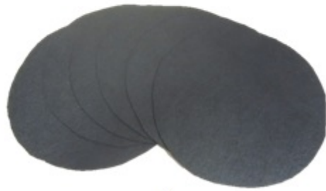
Figure C-2: Sweep test equipment (a) holding pan and brush holder, (b) specimen compactor (c) testing apparatus set-up, and (d) standard asphalt felt disks
