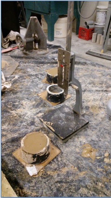
Setting time testing of zero-cement mortar
