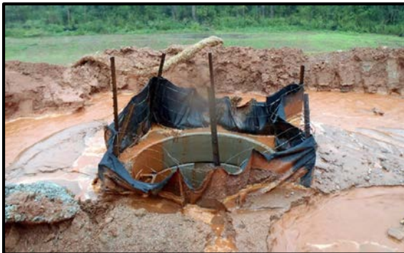
(c) structural failure and flow bypass
