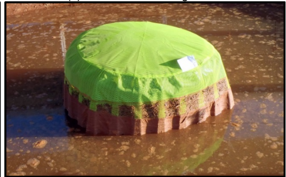
(f) round dome with add'l aggregate disfigurement
