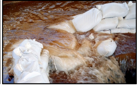
(b) ALDOT standard installation failure
