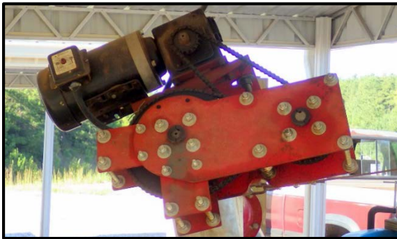
(c) motor, gearbox, sprockets, and chain
